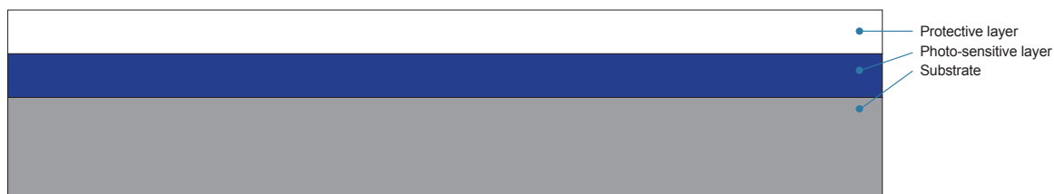
The sketch of CTP photopolymer plate
